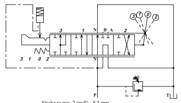
Stroke to pos. 2 (pull) - 8,5 mm Stroke to pos. 1 (push) - 5,5 mm "High force mode" Stroke to pos. 3 (push) - 5,5 + 5 mm "High speed mode"
